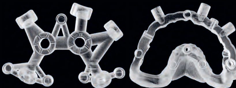
FIGS 23/24 Surgical guides after removal of support material and cleaning.
